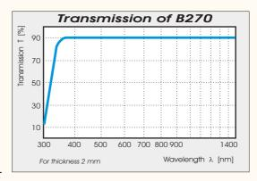
headlights, for clock and display glasses, in photocopiers and oscillographs, binoculars, magnifying glasses and torches, lenses and prisms. Wherever light has to be transferred without undergoing any adverse change, clearly and without obstruction, B270 Superwite® is an important element in solving a problem.
